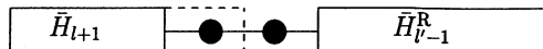
Fig. 2. One step of the finite system DMRG algorithm (left-to-right phase). \tilde{H}_{l+1} and \tilde{H}_{l-1}^R are system block and environment block Hamiltonians in the reduced density matrix eigenbasis.
